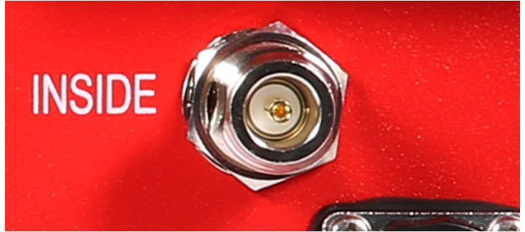
A1 – N-type Female for INSIDE cable and antenna
